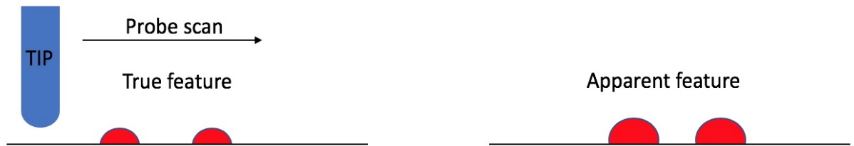
Figure 1.27: Peak broadening of AFM tips. Schematic representation of how tip optimisation for experiments is crucial. If the tip is too big (10 nm) to image the sample (1 nm), the apparent feature of the sample imaged will seem bigger (10 nm) than the one it actually has (1 nm).
