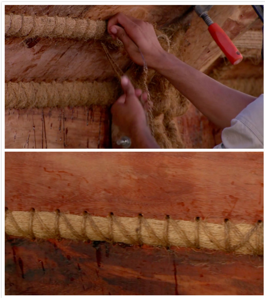
Figure 2.8 Examples of sewing technique
