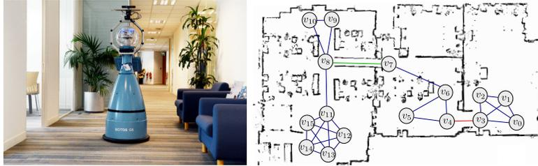
Figure 1: The mobile service robot we aim to use for the demo, deployed in an office scenario (left) and a topological map (right). Edges in blue represent the default laser based navigation, the edge in green represents a specialised ramp traversal behaviour, and the edge in red represents a specialised door crossing behaviour.
