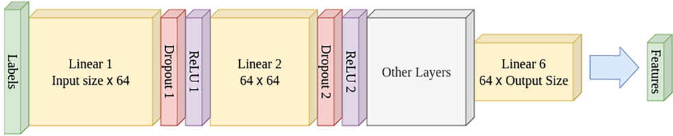
FIGURE 24. Feed-forward neural-network architecture described in Appendix B.5. The layers are shown in the order in which they are applied to the labels. The internal dimensions of the linear layers are 64 \times 64 , whereas the first and last layers match the dimensions of the label and feature vectors, respectively. Dropout layers are included only for local-value predictions. The ‘other layers’ block represents a sequence of 64 \times 64 linear layers, dropout layers, and ReLU layers.
