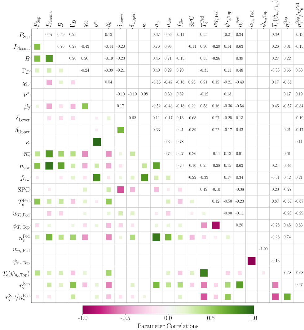
FIGURE 22. Matrix of Pearson correlation coefficients computed for engineering parameters, magnetic-equilibrium parameters, and relevant profile parameters across the database. Here SPC refers to the strike-point configurations, as denoted in Appendix A.1 . The upper triangle contains the numerical values of the correlation coefficients, the lower triangle represents the same values pictorially. Values that are smaller in magnitude than 0.10 are omitted.
