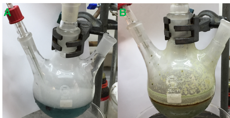
Figure 4 – A) The initial blue colour formed when the bis(acid chloride) is dropped into the ice cold ammonium hydroxide and B) The green solid suspended in brown liquid that appears towards the end of the reaction.
