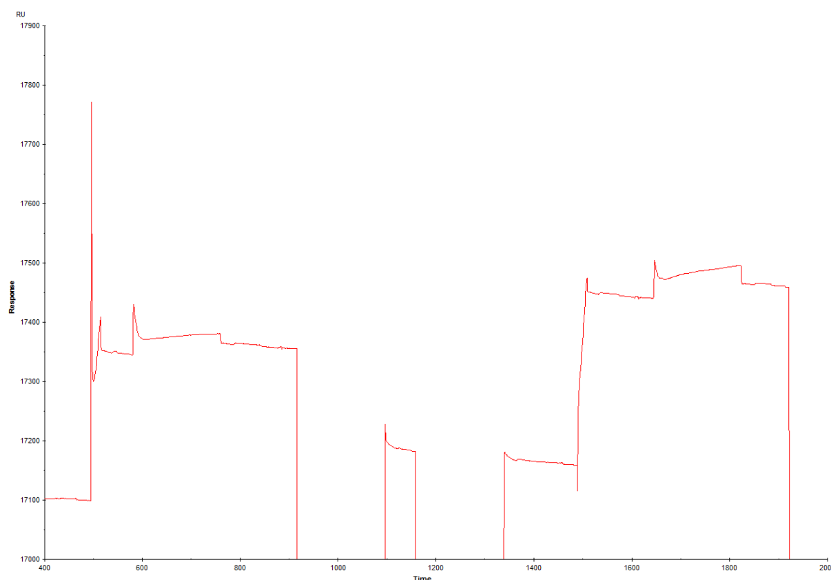
Figure 48 -Noncovalent binding of histones R followed by flowing Sirt2 over the chip and acid wash, repeated with S variant
