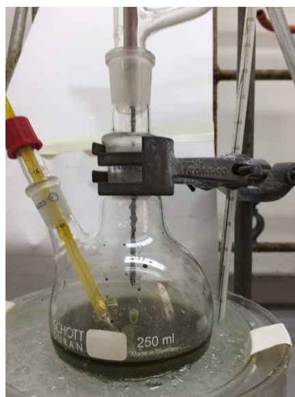
Figure 11 - Stalactite of acid chloride which forms when ammonia vapour is allowed to build up, its eventual collapse leads to a large spike in temperature.
