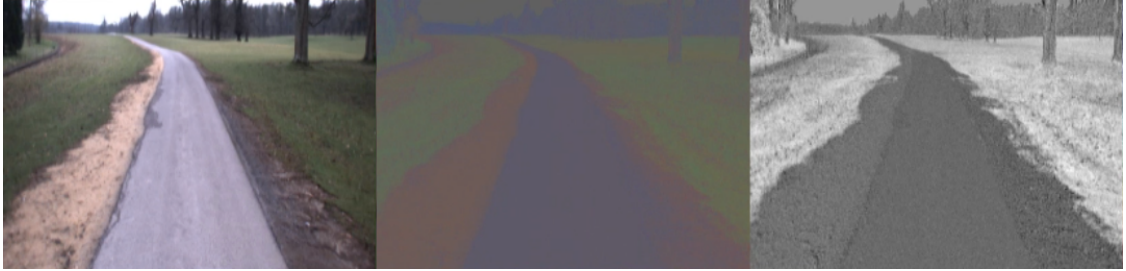
Figure 3.1: Input image (left) and extracted colour channels: RG chromaticity (middle), illumination invariant (right).
