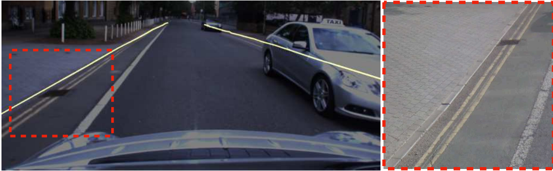
Figure 4.7: The road boundary on the left hand side of the road has no height difference between the road and pavement and it was precisely annotated in the laser pointcloud by simultaneously displaying its projection on the camera image in the annotation tool and using it as a reference while annotating.
