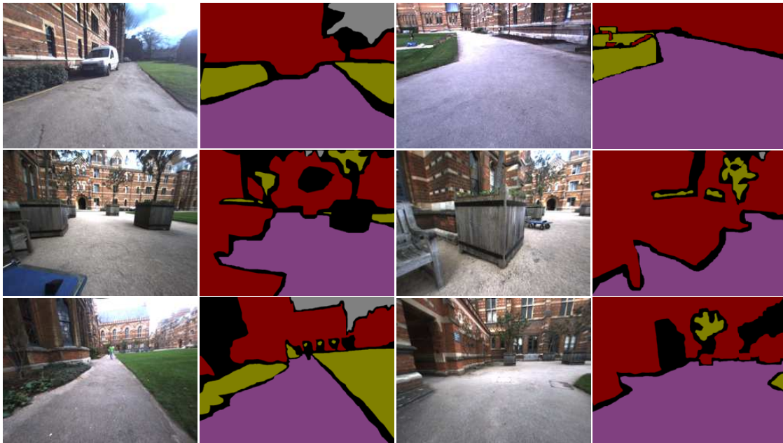
Figure 2.6: Keble College Dataset examples: RGB images with corresponding pixel-wise semantic labels. There are 4 classes: traversable area (purple), vegetation (green), obstacles (maroon), and sky (grey). Pixels in black were not annotated and were not used during the training.
