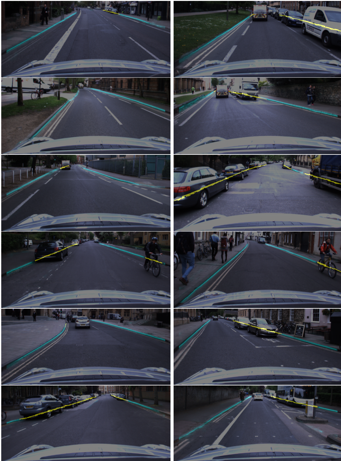
Figure A.1: Camera-based road boundary detection examples. Visible road boundaries (cyan) are detected by the VRBD model, and occluded road boundaries (yellow) are hallucinated by the ORBI model.
