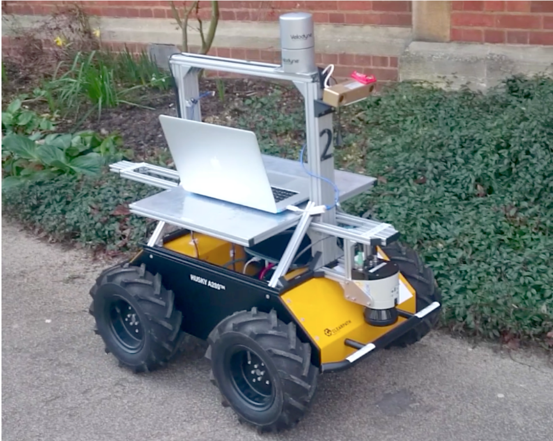
Figure 2.5: Clearpath Husky UGV - the data collection platform for the Keble College Dataset. It has a maximum speed of 1.0 m/s.
