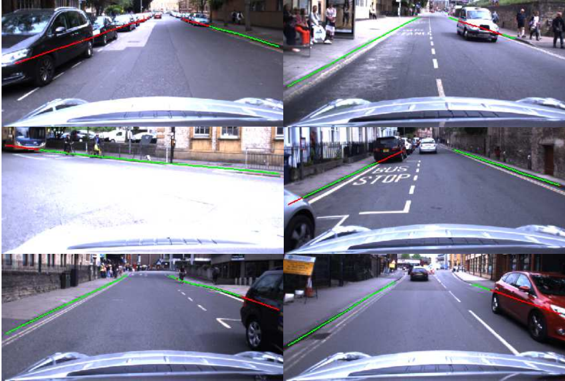
Figure 5.5: Partitioned training data examples with two classes: visible (green) and occluded (red).
