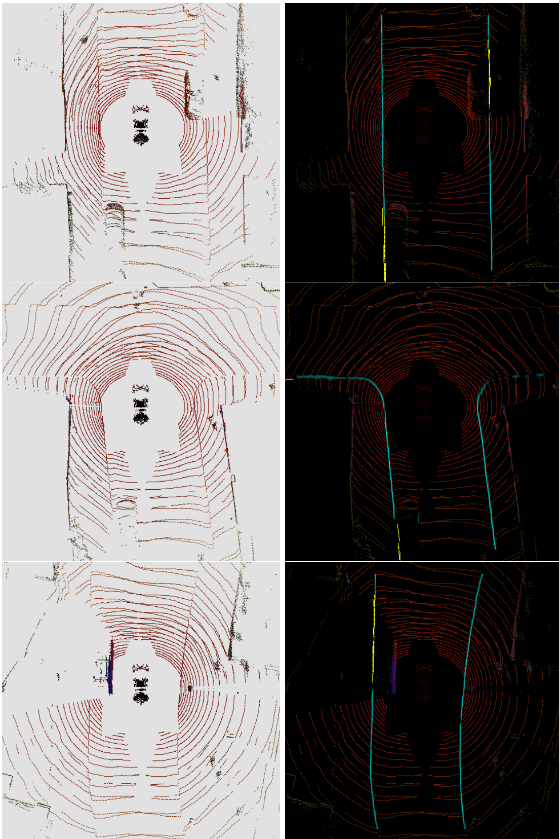
Figure 6.11: Output samples of detected visible and inferred occluded road boundaries by the VRBD and ORBI models with an ROI of 24 \times 24 square metres.
