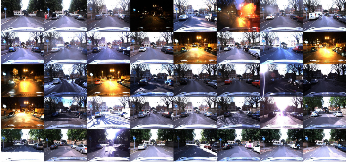
Figure 2.3: The Oxford RobotCar Dataset examples. Each image is a view of the same location from different traversals of a 10 kilometre long consistent route in Oxford City.
