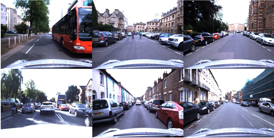
Figure 4.1: Examples of road boundary occlusions: partial occlusion (first column), full occlusion (second and third columns).
