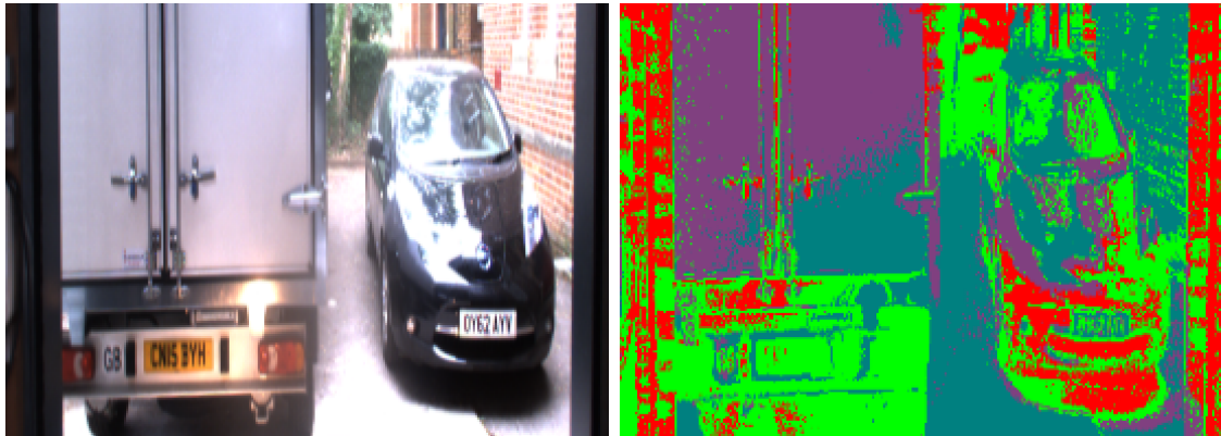
Figure 3.7: Example in which the RF model fails to produce reasonable segmentation in an unusual environment.
