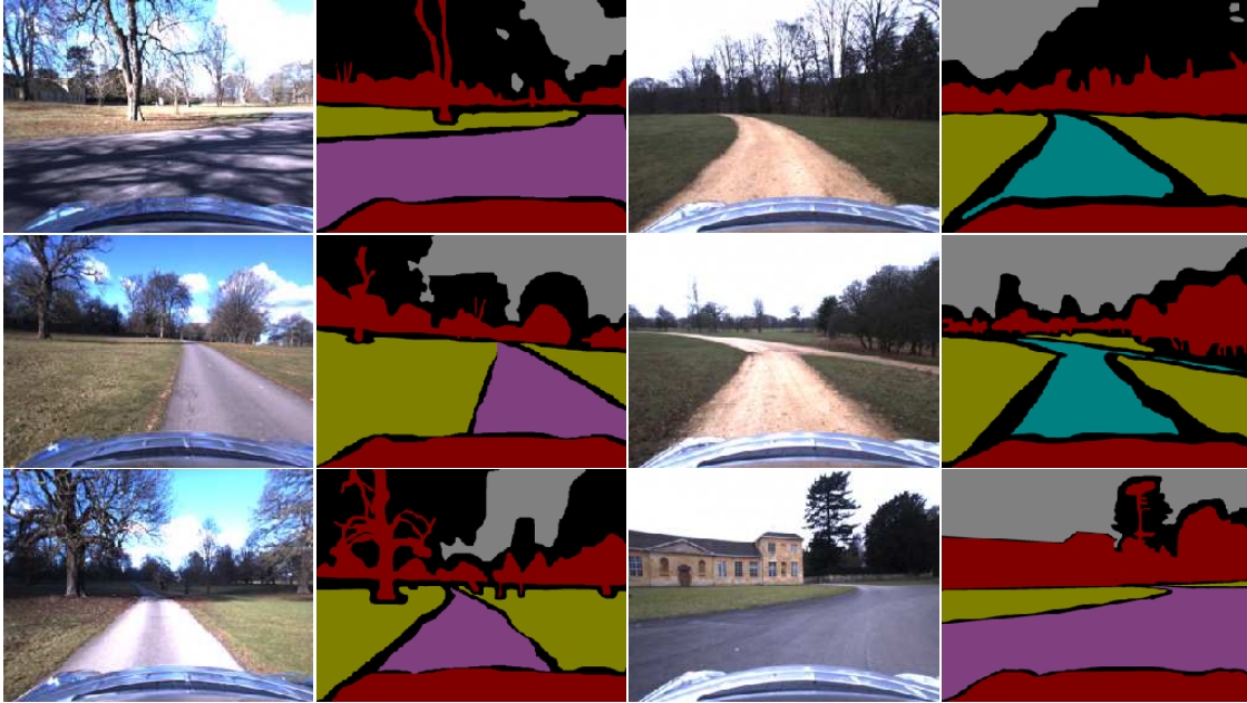
Figure 2.4: Cornbury Dataset examples: RGB images with corresponding pixel-wise semantic class labels. There are 5 classes: tarmac road (purple), dirt road (cyan), grass (green), obstacles (maroon), and sky (grey). Pixels in black were not annotated and were not used during the training.
