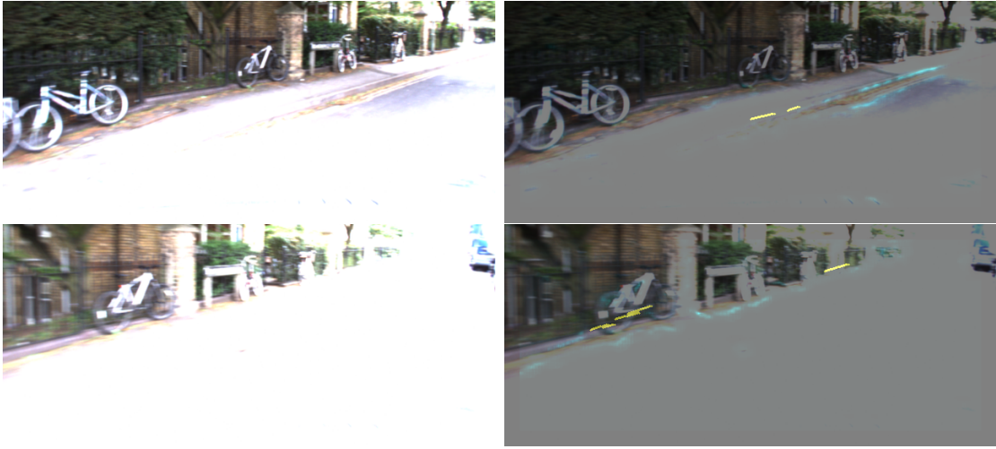
Figure 5.18: Overexposure output samples, where the camera-based models failed to detect road boundaries to a reasonable level.
