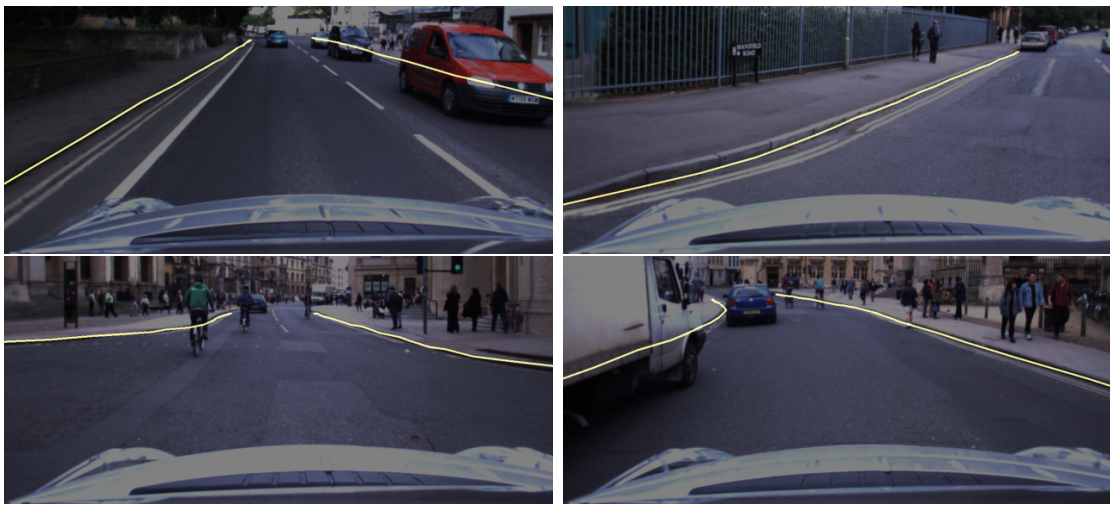
Figure 4.6: Generated “raw” road boundary training data examples: road boundary masks overlaid on top of RGB images. These masks are generated by projecting labels from annotated 3D point clouds into the corresponding images and they contain both visible and occluded road boundaries.
