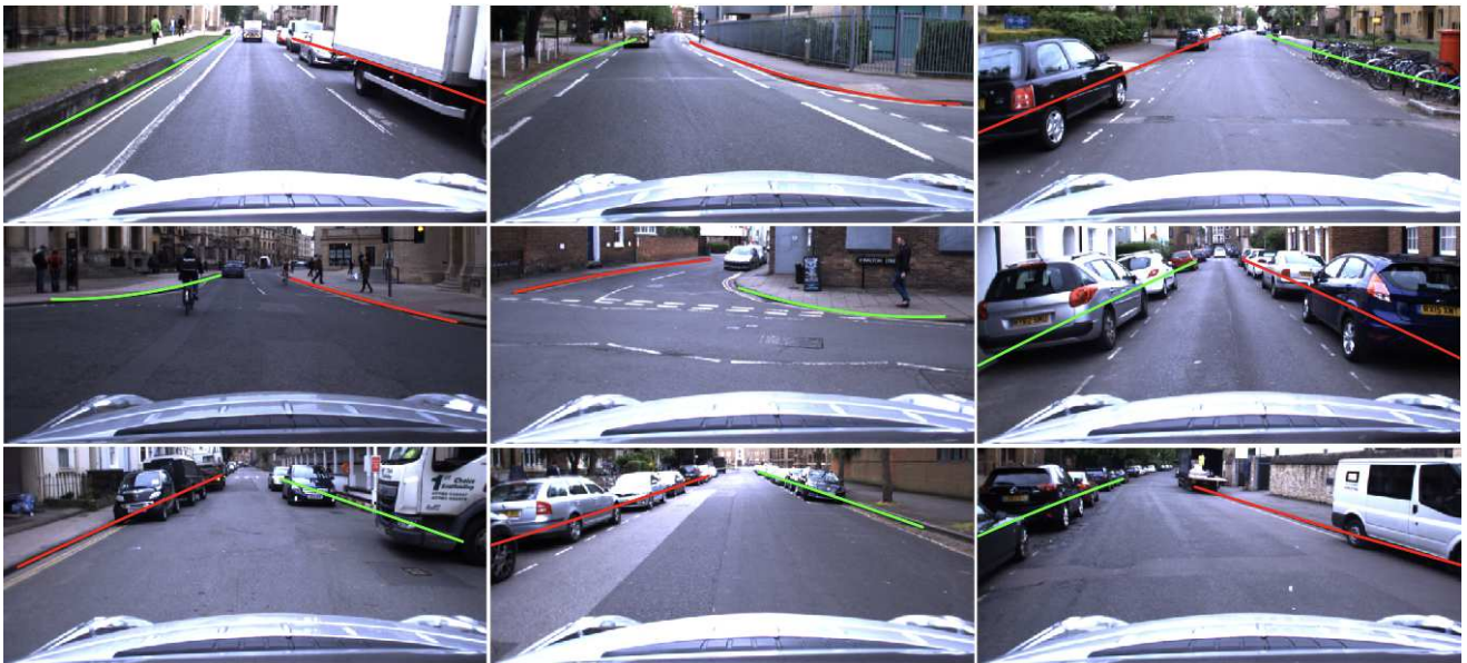
Fig. 11: Sample results of geometric road boundary model extraction from the network output. CORAL is able to obtain the minimum set of cubic curves that represent the road boundaries, without any prior information of the number of models, in a diversity of viewed scenes.
