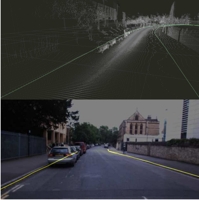
Fig. 2: An annotated 3D point cloud (top) used for generating the training data. Points lying on the same continuous road boundary are given the same ID and lines are drawn between consecutive points to annotate road boundary regions in-between the points. The raw road boundary mask (bottom) is generated by projecting 3D annotations into the corresponding image. The mask contains both visible and occluded road boundaries.
