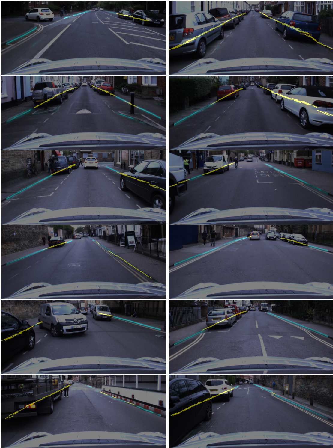
Figure A.2: Camera-based road boundary detection examples. Visible road boundaries (cyan) are detected by the VRBD model, and occluded road boundaries (yellow) are hallucinated by the ORBI model.
