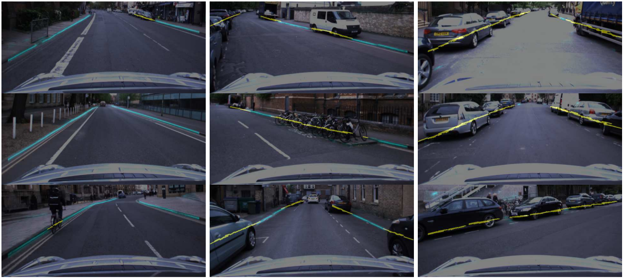
Fig. 10: Sample outputs from the network under different levels of road boundary occlusion. The network is able to seamlessly deal with and predict the position of the road boundaries in scenarios of low to no occlusion (left column), some occlusion (middle column) and full occlusion (right column). The blue pixels are the visible road boundaries while the yellow pixels represent the occluded boundaries.
