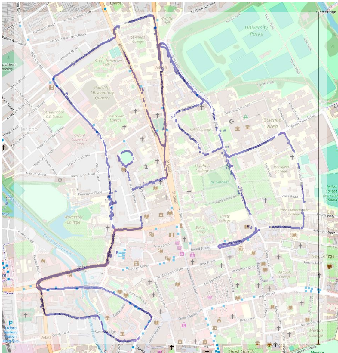
Figure 6.13: 31100 samples of the 18-01-19 dataset are overlaid on a digital map using GPS coordinates. Although the dataset is a complete loop, we observe many gaps along the route.
