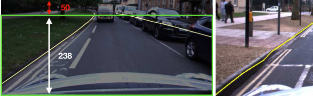
Fig. 9: Left: the area inside the green box is taken into consideration during the evaluation. Right: the width of the ground truth curb line is always the same regardless the height of the curb.
