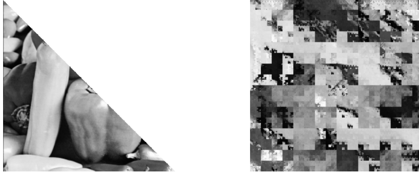
Figure C.11: An example of the encoding map taking data from a triangular domain and mapping it to an array of each ‘triangular pixel’ value under lexicographical ordering.
