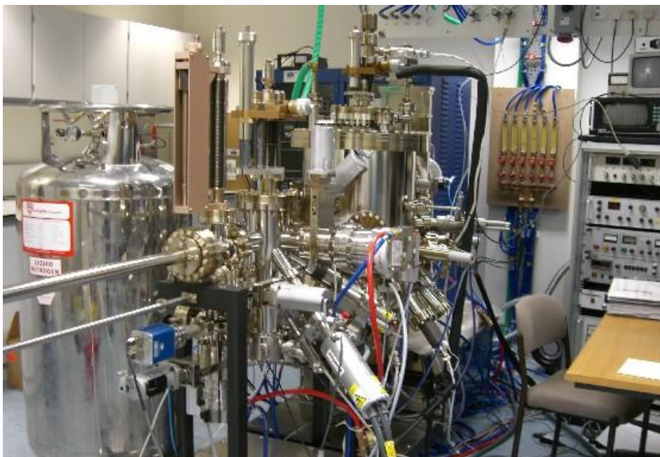
Figure 3.1. The setup of the oxide MBE system at Oxford (Photo taken by R. G. Egdell).
