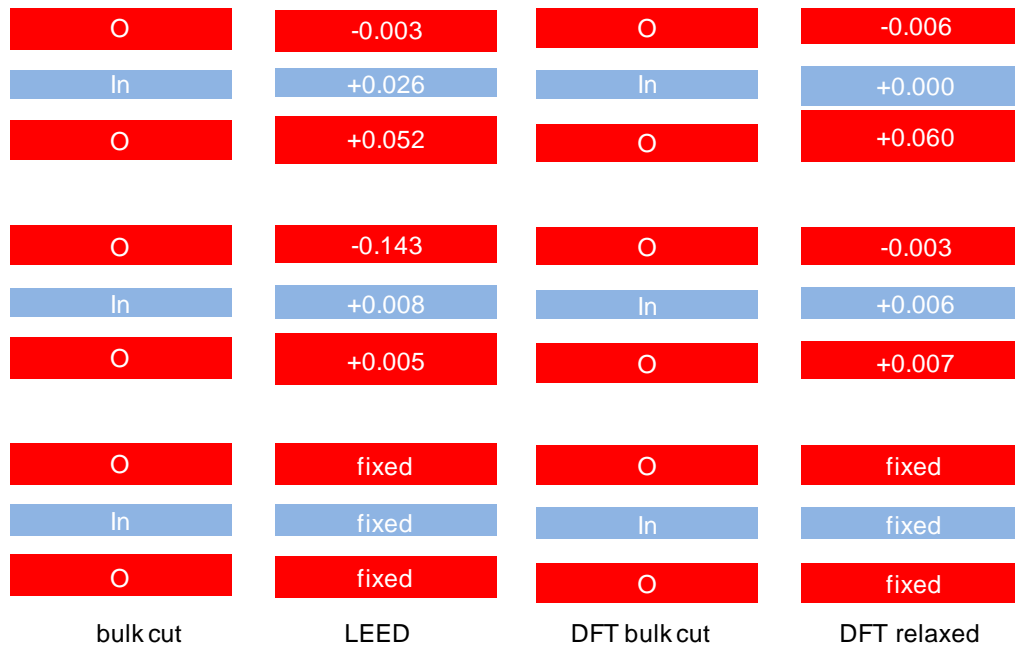
Figure 6.8. Schematic representation of the structure for \text{In}_2\text{O}_3(111) derived from truncation of the bulk structure and from analysis of LEED I/V data. Comparative diagrams for a bulk cut DFT structure and a relaxed DFT structure are also shown. Owing to the complexity of the structures individual atomic positions are not shown but the spread of atomic positions within components of the quadrupolar layers that are characteristic of the (111) surface are represented by the width of the horizontal stripes. The numbers inside the stripes give the straddle of atomic positions within a layer (in Å), while the figures in parentheses for the LEED and relaxed DFT structures give the average vertical relaxation of the atoms within a given layer (also in Å). Positive numbers refer to inward relaxation; while negative refer to outward relaxation.
