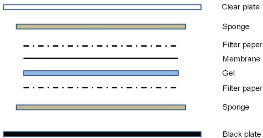
Figure 46. 'Transfer sandwich' used for transfer of protein from SDS/polyacrylamide gel to a polyvinyl difluoride membrane.
