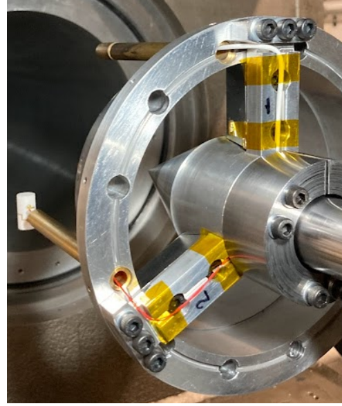
Fig. 8: Photograph from shot T6s333 showing sensor wires taped into channels in the ring mount.
