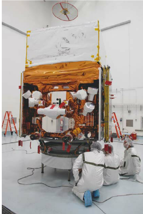
Figure 1.1: The Fermi space telescope on Earth, with its solar arrays folded. LAT is the block at the top of the satellite covered with the silver anti-coincidence shield. GBM consists of the cylindrical structures protruding from the lower half of the telescope. Note the size of the engineers relative to the size of the instrument, this highlights the comparatively small effective area of LAT. Image credit: NASA/Kim Shiflett.
