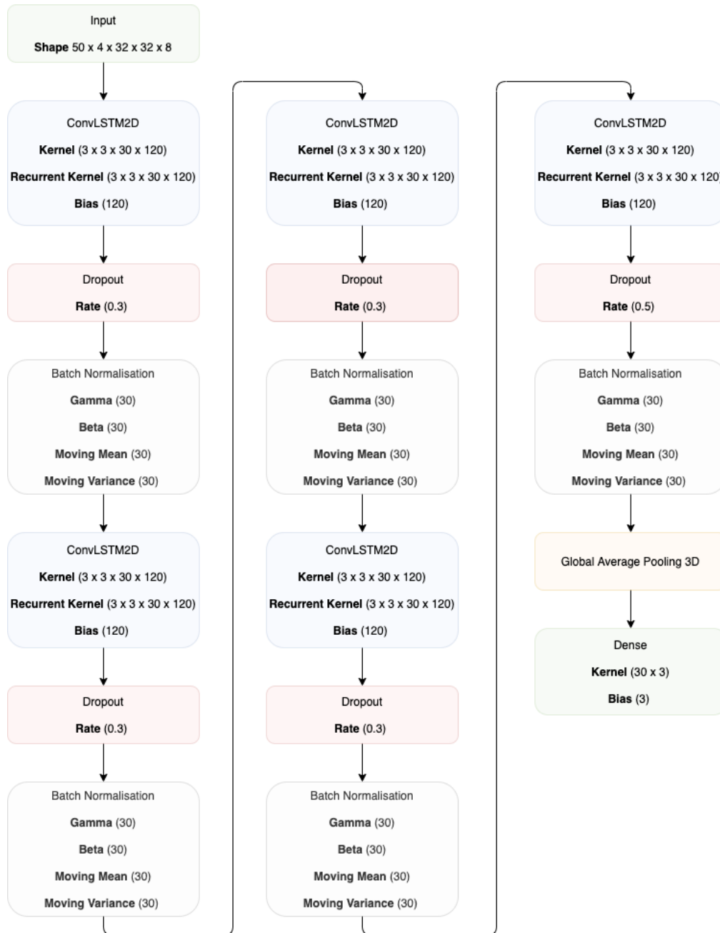
Figure 3.5: Example of our CNN-based ConvLSTM2D architecture. The only difference between the various methods A-D was the shape of the input vector, as some methods used more pixel maps than others.
