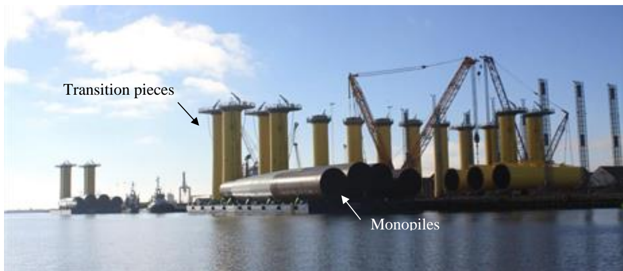
Figure 1.9 Current largest monopile installed ( D = 7.5 m) at the Gode Wind Offshore Wind Farm in the German North Sea (Figure from DONG Energy, 2015 6 )
