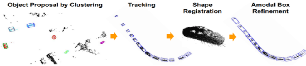
Figure 4.6: Flow diagram of DBSCAN++.
