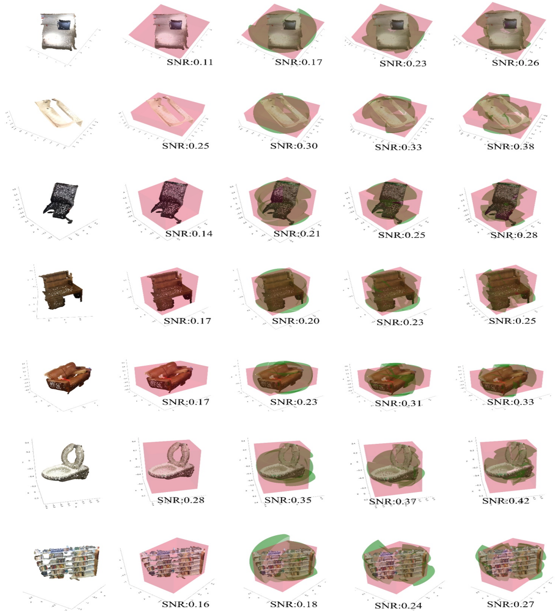
Figure 3.12: Visually comparing AABB and RID with different configurations of N_\theta and N_\phi for various instances, such as bed, bathtub, chair, desk, sofa, toilet, and bookshelf. A larger signal-to-noise ratio(SNR) means fewer background points inside the coarse detection, leading to higher precision for the refinement stage and thus improving the overall system performance.
