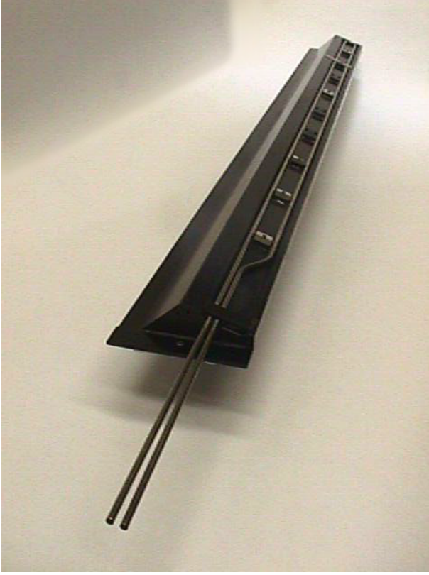
Fig. 11. Bare support structure for barrel modules
