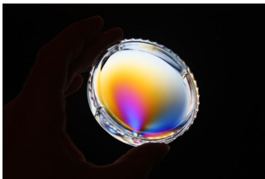
Figure 2.19 Residual stresses in an injection moulded plastic disc (open source image-Zephyris)
