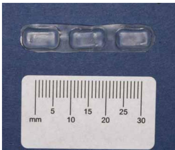
Figure 2.12 “Fabricated tissue expander devices: coated, subunit 8 x 4 x 1mm”. Image reproduced from (6)
