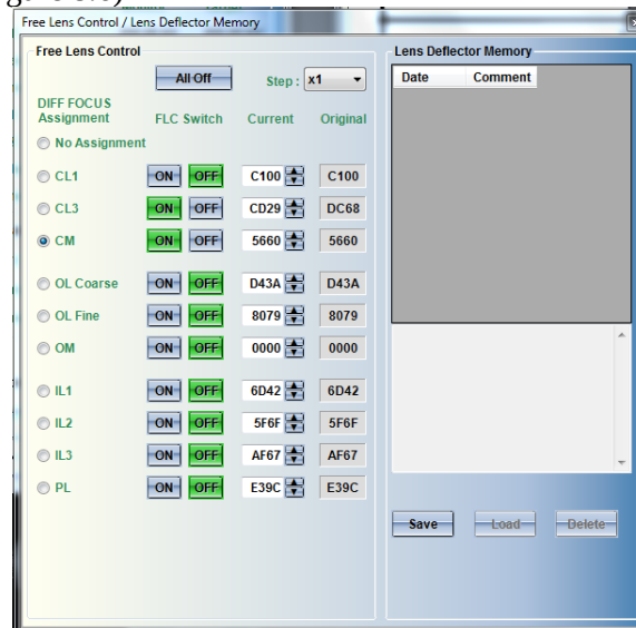
Figure 8.6 Free Lens Control (FLC), CL3 should be switched on in mag mode, whereas Cm should be switched on in alignment mode.
