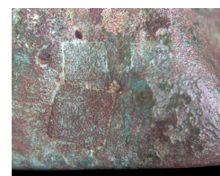
Figure 4.26. Casting patches on cat 196 , to the left of the tail.
