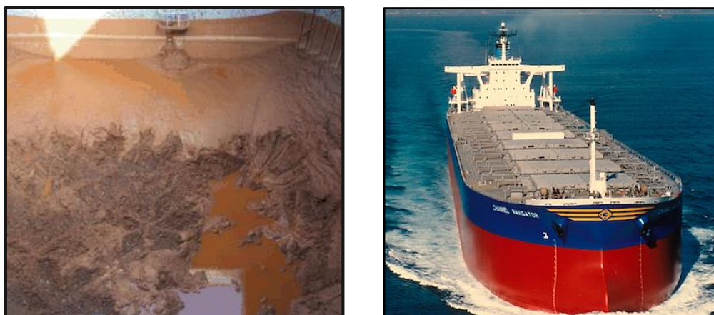
Figure 1.1: (a) What is considered to be liquefied cargo within a ship’s hold (Grant, 2008) (left); and (b) a Capesize solid bulk carrier (Golden Ocean, 2014) (right).
