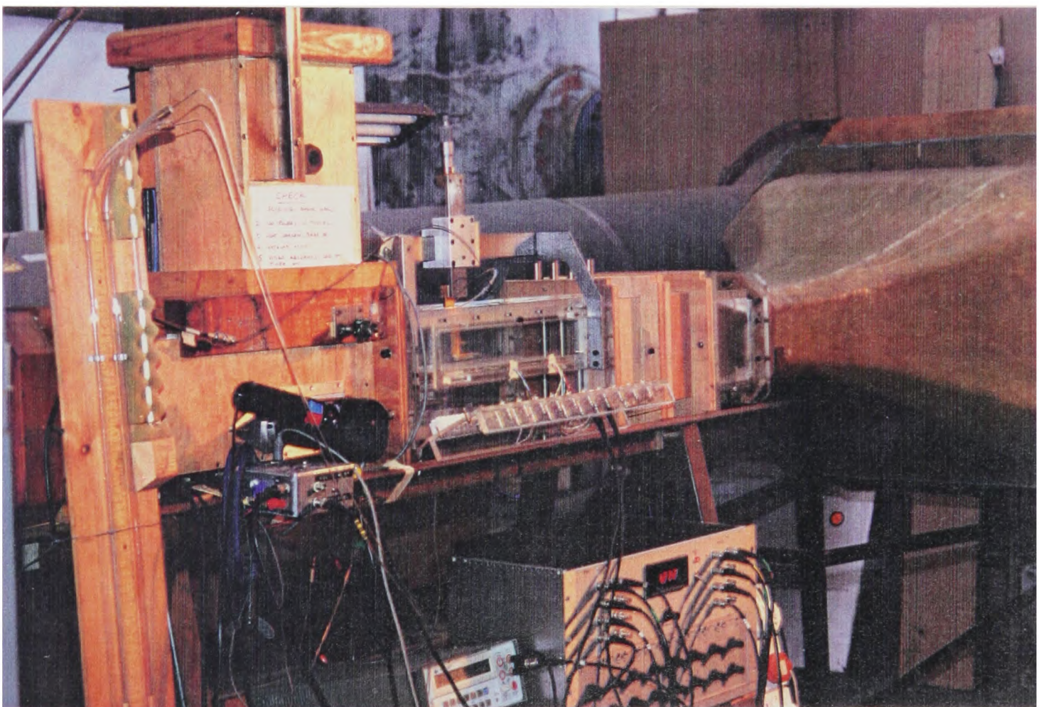
Figure 5.4. Photograph of working section used for the flat plate heat transfer experiment. This was used for both the liquid crystal tests (perspex plate) and the thin film gauge tests (Macor plate).
