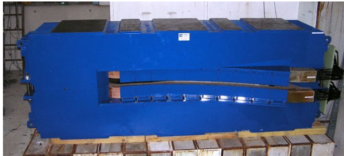
Figure 2.6: The RACCAM spiral FFAG prototype magnet. Image courtesy of LPSC Grenoble.
