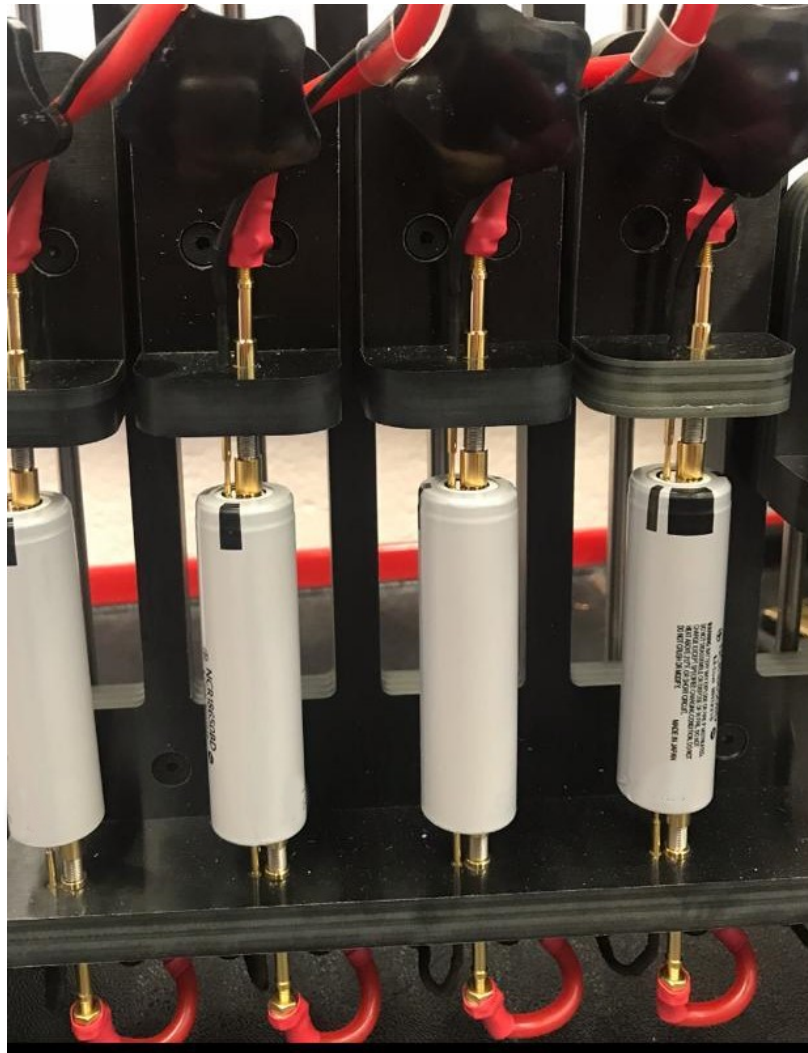
Fig. 2.5 Four terminal spring loaded cell holder
