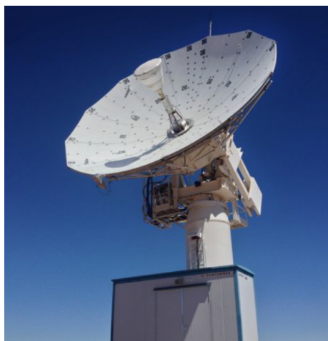
Figure 3.12: C-BASS South in operation Klerefontein, South Africa. The photogrammetry targets are visible on the twelve panels that make up the primary reflector and the foam cone supports the secondary mirror on top of the receiver (Taylor (2018)).
