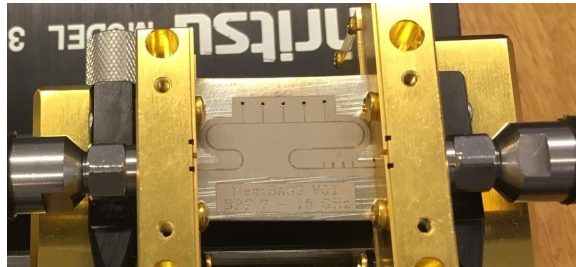
Figure 5.19: The 7-15 GHz bandpass filter realised in micro-strip.
