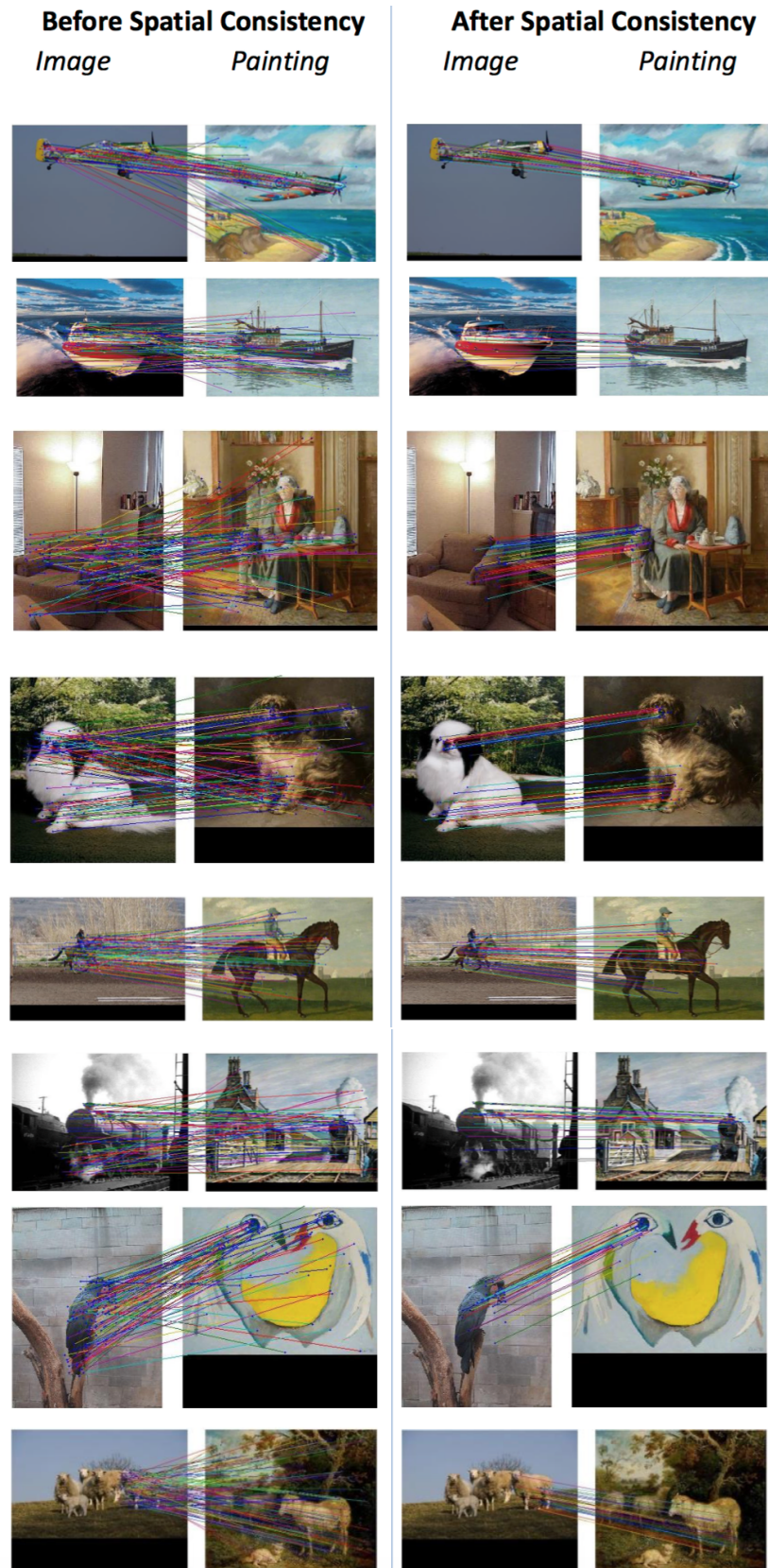
Figure 4.2: Image-painting pair correspondences before (left) and after (right) computing a spatially consistent subset. Note, that the MLDP correspondences are able to generalise slightly over viewpoint, intra-class differences, and between natural images and paintings.
