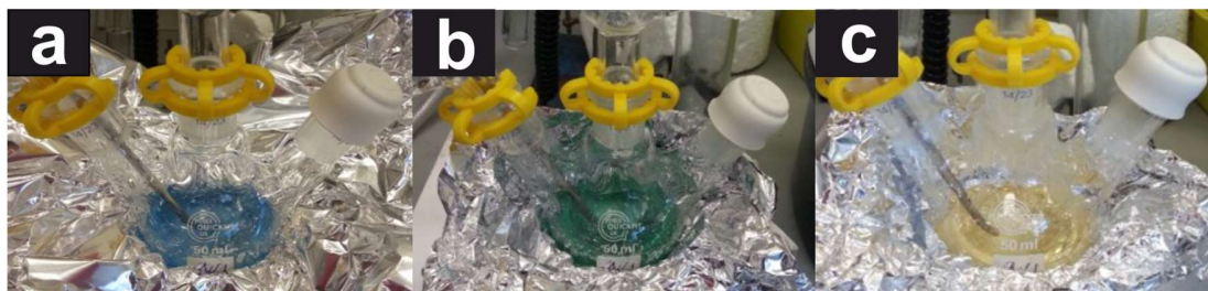
Figure 25- Showing colour change in the solution with increasing reduction temperature. From 30°C to 130°C, colour changes from blue → green → yellow, indicating that Cu has been fully reduced.
