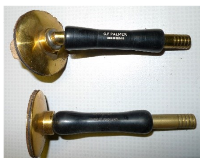
Figure 6.3 Palmer kymograph fittings preserved at Oxford University Phonetics Laboratory (cf. Figure 6.2). From top: speech tambour, mouthpiece (note the relief valve), nasal olives in three sizes, angled and straight larynx capsules. Photographs: the author.
