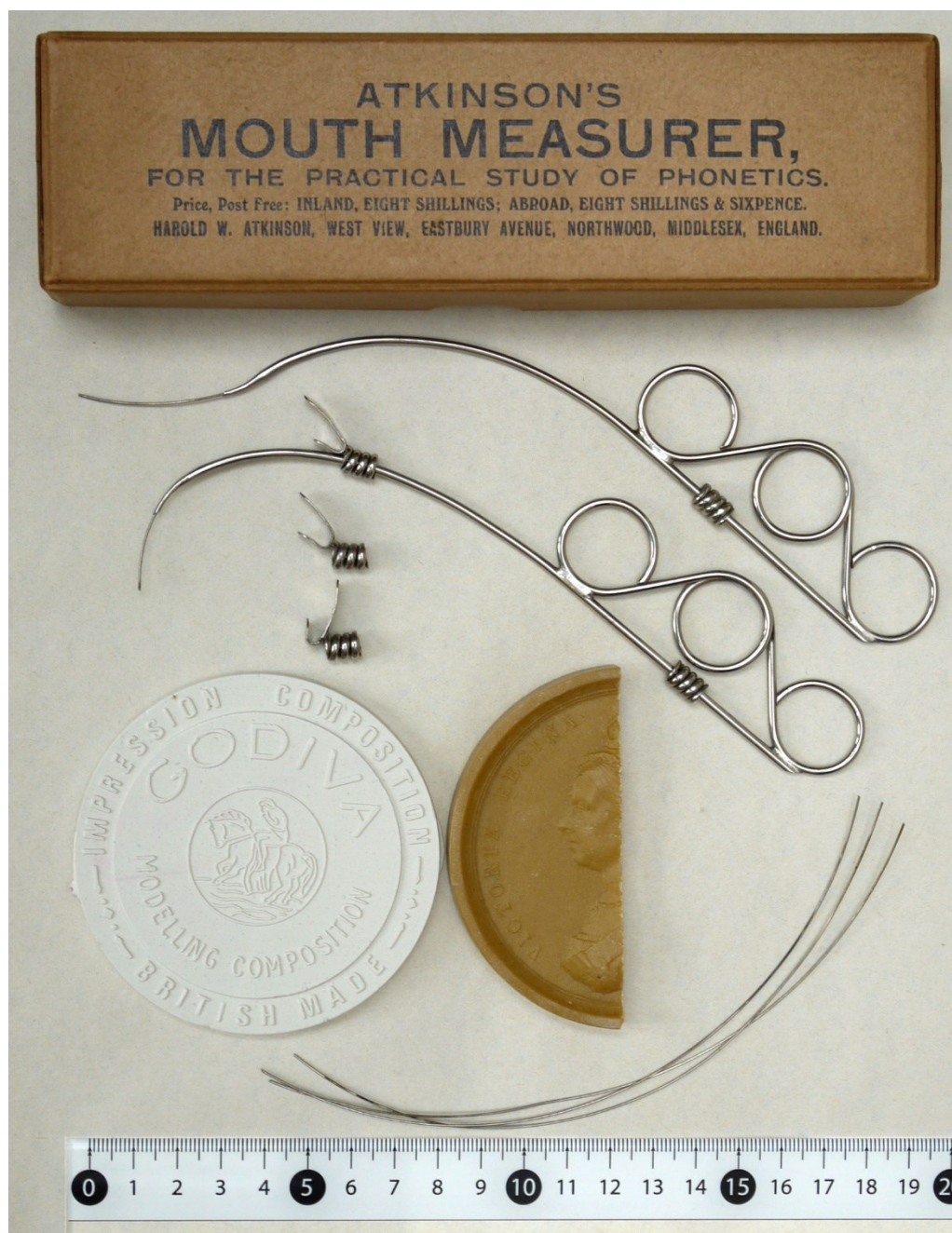
Figure 2.15 Atkinson's Mouth Measurer as supplied in its box. The instruments were in pairs. In one (upper) the probe wire emerges with an upward curl (towards the palate), and in the other downwards (towards the tongue surface). A selection of tooth stops was supplied with differing angles; they can be further tailored easily by bending. The half disc is exactly 1 oz. of modelling compound, supplied for making a (partial) cast of the palate. It is the same diameter as the modern disc of Godiva shown next to it and precisely half the weight. Replacement probe wires were also included.
