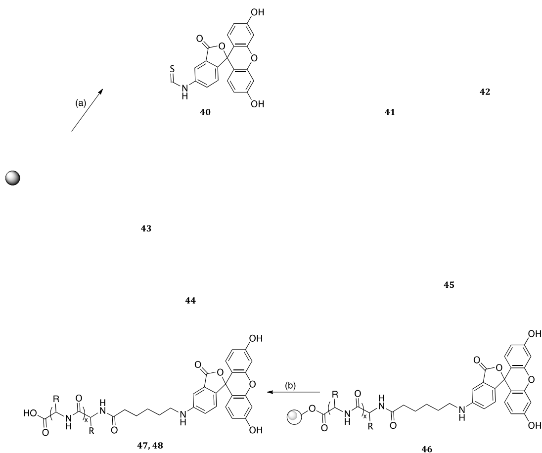
Figure 2.32 – General scheme for the formation of a fluorescein thiohydantoin and the synthesis of FITC labelled ER-retaining peptides. Reagents and conditions: (a) FITC, DIPEA; (b) TFA; (c) HOBt, DIC; (d) 20% piperidine in DMF.
