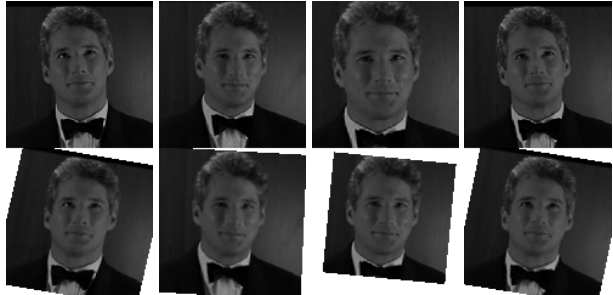
Figure 2: Affine registration. (Top) Sequence of faces obtained by the face detector. (Bottom) Affine registered sequence. There is an overall unresolved affine transformation which must be accounted for when comparing this with other such sequences.
