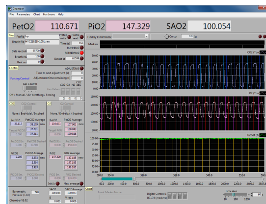
Figure 2.8 The operation window in Chamber software The status of the system is on the left side. The right side shows participant's P_{O_2} trace, P_{CO_2} trace and oxygen saturation (from top to bottom) in a 1 minute period.
