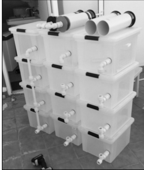
Figure 4.2. Photograph of the FRS translocation containers, showing the PVC filters and piping to draw flow through the containers. The left-most stack is fitted with the tubing in parallel ready at the negative pressure (vacuum) end. Headtorch for scale.
