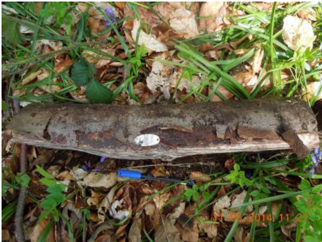
Figure 2 One beech log with an aluminium tag attached by an aluminium wire placed in a beech dominated canopy area.
