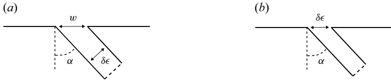
Figure 16. Angled geometry with (a) constant branch width \delta\epsilon and hole width w , and (b) constant hole width \delta\epsilon . The angle, \alpha , is defined between the branched channels walls and the negative y-axis.
