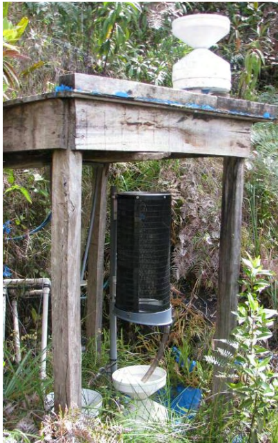
Figure 6.2. The cylindrical fog-interceptor installed with the permanent weather station at the Wayqecha research site.
