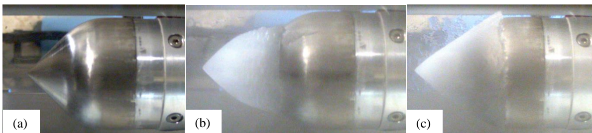
Fig. 10 (a) Clean 45^\circ half-angle test piece. (b) Accretion corresponding to Fig 9(b) at test completion, M = 0.25 , MR = 12.5\% , PSD 2. (c) Accretion at test completion for a run at M = 0.40 , MR = 9.3\% , PSD 2.
