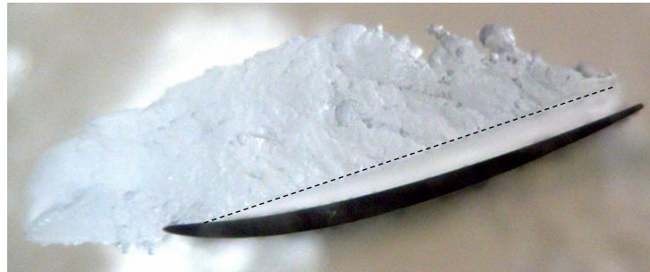
Fig. 7-25 Run TR814 after the cloud was switched off, after ~ 180 s of exposure. The contact surface between accretion and aerofoil before rotation is shown by the black dashed line.
