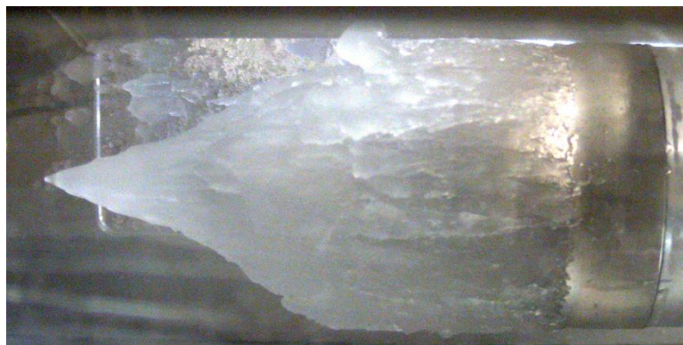
Fig. 7-16 Accretion on the 20° cone for M = 0.25 , D_{v50} = 34 \mu\text{m} and MR = 0.11 after ~ 240 s of exposure
