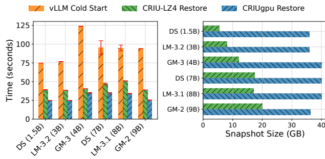
Figure 7: vLLM cold-start latency, CRIU-LZ4 and CRIUgpu restore times (left) and snapshot sizes (right) for vLLM containers serving Gemma (GM), LLaMA (LM), and DeepSeek-R1 (DS) models. The container rootfs and checkpoint image files are stored on a local in-memory filesystem.
