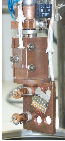
Figure 2.24: A DLTS specimen in the specimen chamber.
