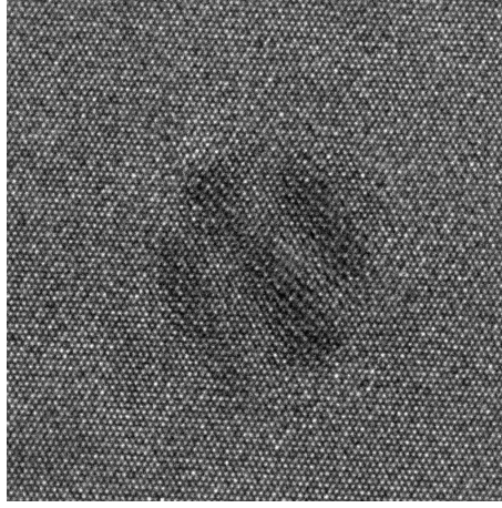
Figure 4.10: TEM micrograph of a precipitate in the bulk of FZ-Si with a nitrogen concentration of 7 \times 10^{14} \text{cm}^{-3} . The as-grown specimen was annealed in an argon atmosphere at 900^\circ\text{C} for 10 minutes (courtesy of Dr K. Jurkschat).
