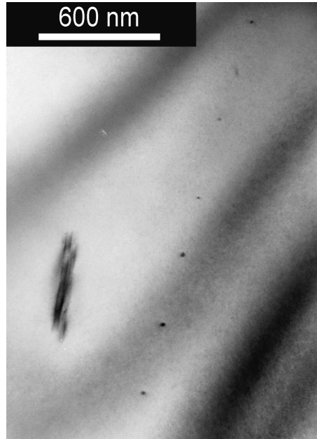
Figure 4.9: TEM micrograph of a line of precipitates in FZ-Si with a nitrogen concentration of 2.2 \times 10^{15} \text{cm}^{-3} . The specimen was annealed at 750^\circ\text{C} to be in regime 2 of dislocation locking and had been subjected to a three-point bend to unlock the dislocations from the pinning impurities (courtesy of Dr S. Lozano-Perez and Dr A. Giannattasio).
