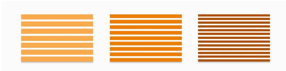
Figure 55. Schematic to illustrate deposition power is inversely proportional to deposition rate.
