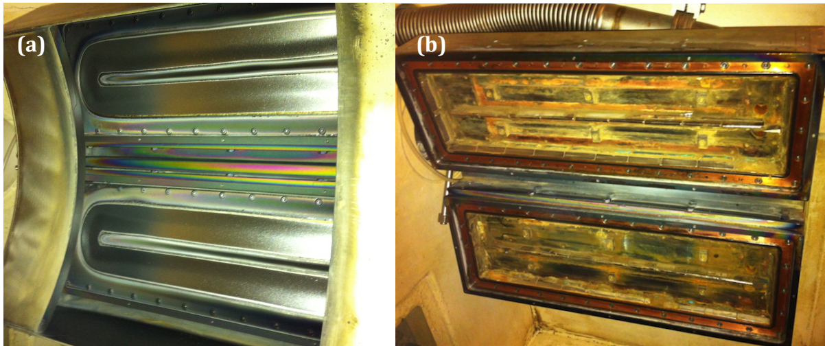
Figure 31. Sputter cathodes of the Oxford Webcoater: (a) the aluminium cathodes exhibiting the sputter wear "racetrack", (b) the aluminium cathode removed, revealing the array of permanent magnets characteristic of a magnetron system.
