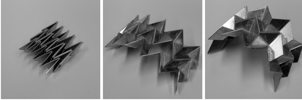
(b) Folding sequence of aluminium prototype
