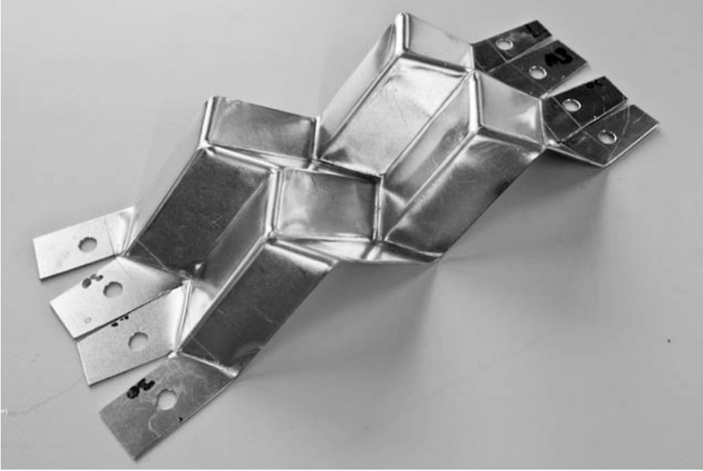
Figure 3.25: Standard foldcore constructed with t_p = 1\text{mm} aluminium sheet.
