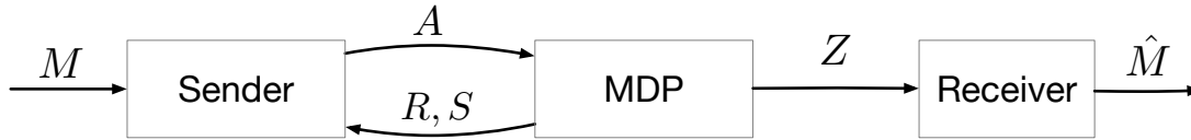
Figure 6.2: Graphical representation of an MCG. First, the sender is given a message. Second, the sender is tasked with a MDP, unrelated to the message. Third, the receiver observes the sender's trajectory. Fourth, the receiver guesses the message.
