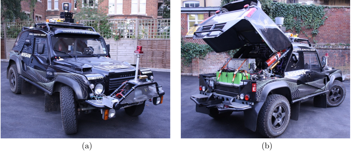
Figure 4.7: Our Wildcat autonomous survey vehicle with which we collected data at night. The omnidirectional Point Grey Ladybug2 (LB2) camera is can be seen mounted in an elevated position at the front of the vehicle. The downward-facing Bumblebee2 camera is mounted next to it. The compute server to which data are logged is visible in the rear compartment.
