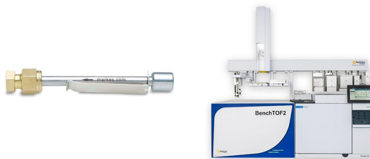
Figure 3.4: Thermal desorption tube from Markes International (left) and two-dimensional gas chromatography (GCxGC) system coupled with a time-of-flight mass spectrometer (TOF-MS) from SepSolve Analytical (right).
