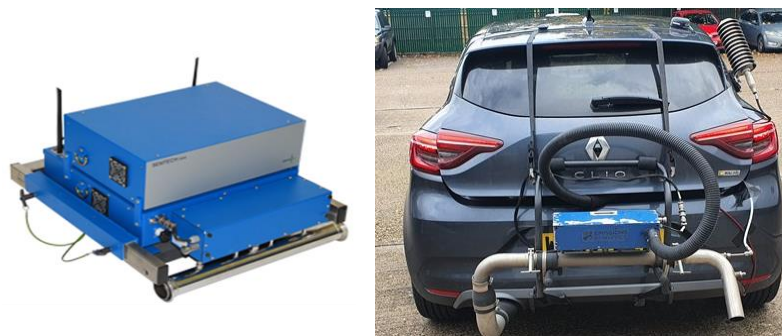
Figure 3.3: SEMTECH-LDV portable emissions measuring system (PEMS) (left) and an example vehicle with the PEMS experimental measurement set-up (right) adapted from [196] with permission from SAE International.
