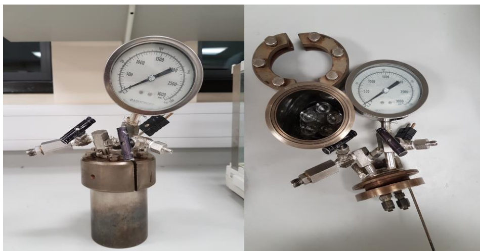
Figure 4-2: The Parr high-pressure system. The system was harder to assemble compared to the Tinyclave, but higher pressure ( > 10 bar) can be applied to the reaction mixture.
