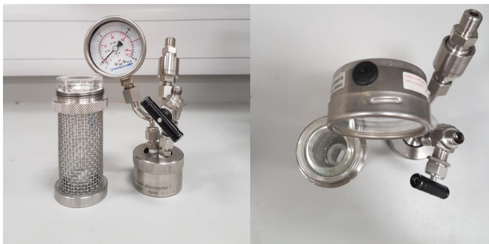
Figure 4-1: The Tynclave apparatus used for alkane oxidation under a total pressure below 10 bar.
