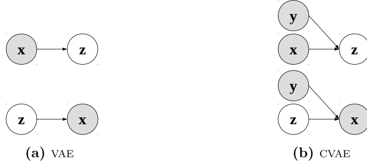
Figure 4.1: Structure of recognition (top row) and generative (bottom row) models for VAE and CVAE. Here, \mathbf{z} denotes the unobserved latent variables and \mathbf{y} denotes the conditioning variables.
