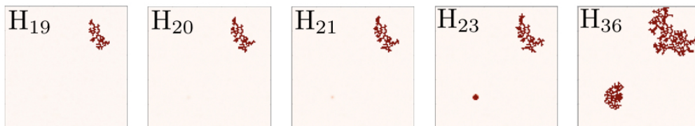
Figure 4: Activation dynamics for weights close to the optimal solution ( \lambda = \lambda_c - 0.227 ). Up to layer 19 ( H_{19} ) the On activations spread according to BFS however at H_{20} a very faint localized unwanted On activation begins to develop (a bug) and quickly saturates ( H_{23} ). Past this point BFS dynamics continues normally but spreads both the original and the unwanted On activations. While not shown explicitly, On activations still appear only on black maze cells. Notably the bug developed in rather large black region as can be deduced from the large red region in its origin. See also a short movie showing the occurrence of this bug at https://youtu.be/2I436BVAvdM and more bugs at https://youtu.be/kh-Af0o4TkU . At https://youtu.be/t-_TDkt3ER4 a similar behavior is shown for the checkerboard-BFS.
