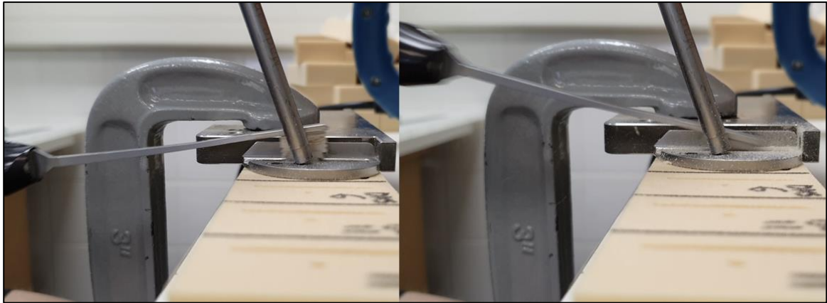
Figure 6.10 Images of how the keel slots were prepared using the Standard Sawblade.
