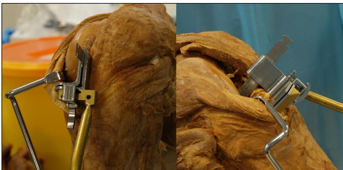
Figure 6.4 The prototype drill bit resection guide in use on a left cadaveric knee (Left: anterior view, Right: Lateral View).
