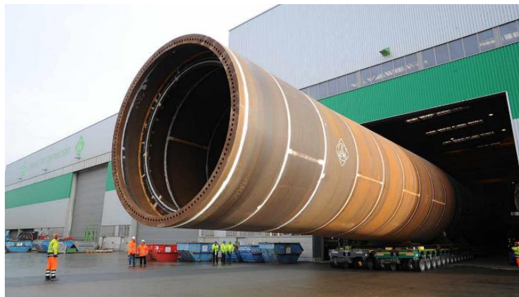
Figure 1-3 Monopile foundation ( D = 7.5 m) for the Veja Mate offshore wind farm (EEW, 2022).
