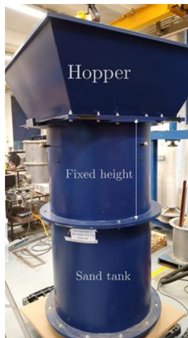
Figure 3-2 Photographs of the sand tank and sand rainer.
