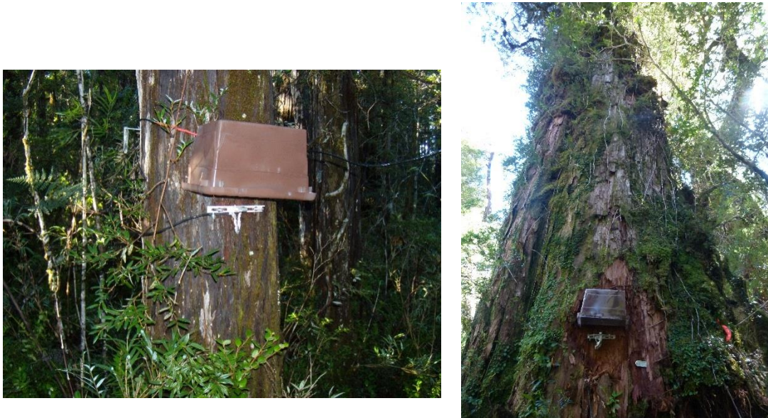
Figure 3.10. Automatic point dendrometers installed in Fitzroya trees from the Coastal (left) and Andean sites (right, Photos: Aldo Farías and Yadvinder Malhi).
