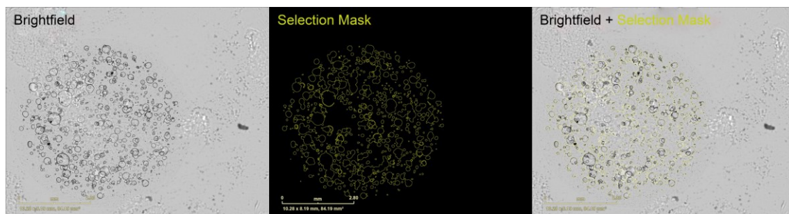
Figure 17. Incucyte® methods to study organoid count, mean area and confluence. (A) With the Incucyte® ‘Whole Well’ module, organoids are hardly visible – image processing enables accurate segmentation analysis. (B) With the organoid module, segmentation can immediately be performed.
