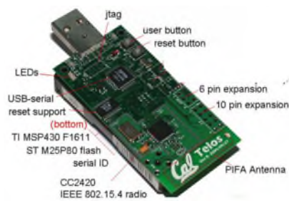
Figure 7: Example of a node, the TELOS platform. The node, excluding battery and packaging, measures 65 x 31 x 6 mm and weights 23 grams. It has a maximum transmission power of 1mW. Image: Polastre et al., 2005.
