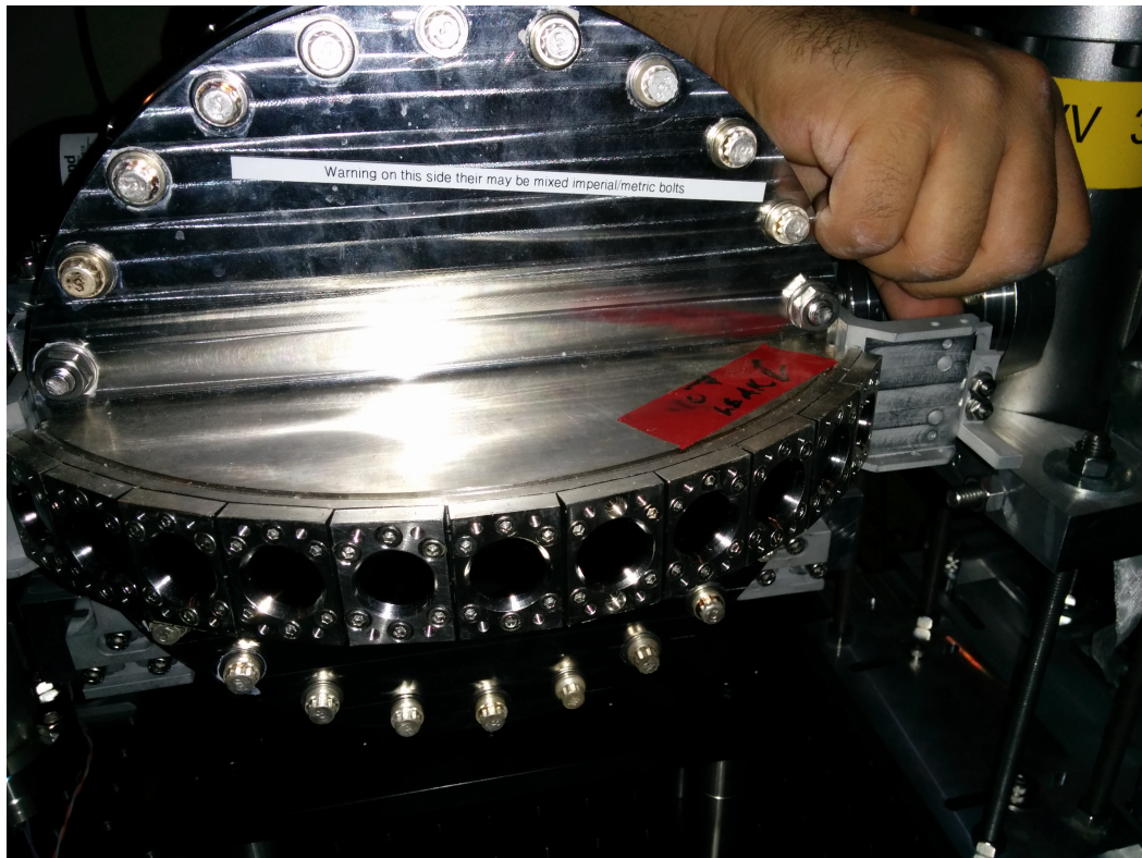
Figure 4.4: The vacuum chamber with its 11 silicon windows, during a hardware operation I undertook with a SLAC technician (Juan Cruz, on the photo)
