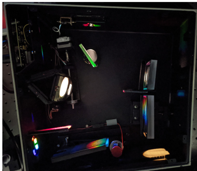
Figure 2.8: The inside of the monochromator, showing the white light split into a spectrum.
