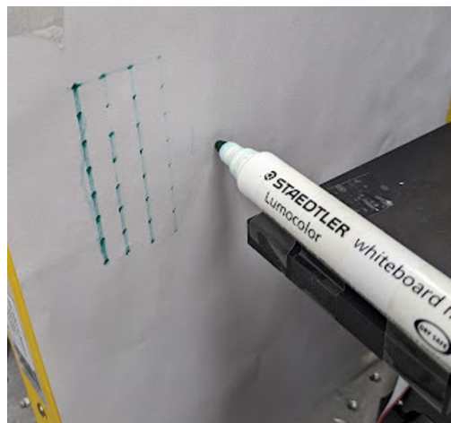
Figure 2.24: The 2D scanning of the linear stage was verified using this simple method of a pen being traced along a piece of paper.
