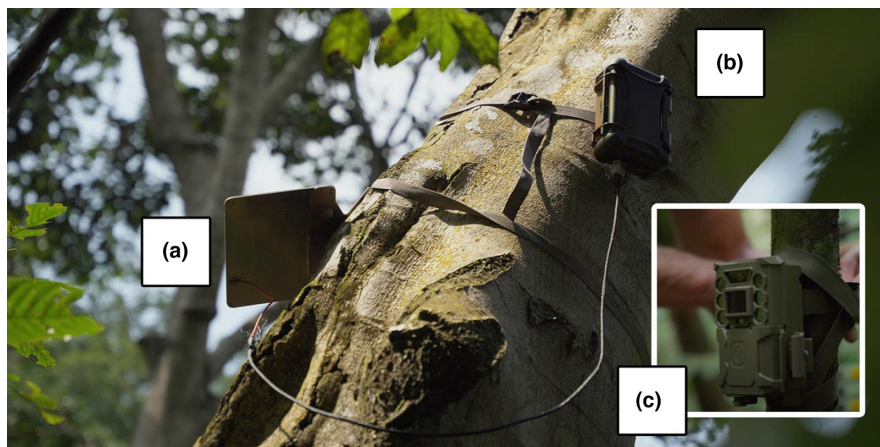
FIGURE 1 System deployed in the field showing (a) the solar panel and (b) smart bridge attached to a tree approximately 6 m above ground level. The Bushnell™ camera trap (c) is installed approximately 40–50 cm above the ground level and approximately 10 m away from the smart bridge.
